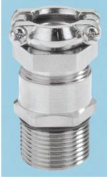
The SKINDICHT® SKZ a double cleat strain-relieving cable gland equipped with a centre section. The arrangement of the double cleat provides a wide clamping range with central cable clamping. The seal is achieved by a recessed sealing ring and an O-ring fitted onto the connecting thread. This cable gland is particularly suitable for use in plugs, switches and control panels.
