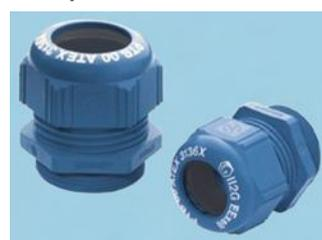
SKINTOP® K-M ATEX is a special cable gland, made of polyamide. It is designed for use with electrical equipment in areas with risk of explosion which require class "e" security. (DIN / EN 50014 and DIN / EN 50019).
