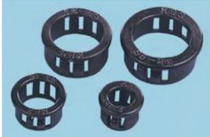
A ridged black Nylon 66 bush. Push fitting to protect and insulate holes in metal chassis. To fit panel thickness 0.8mm to 3.2mm. Flame retardant to **UL94V-2**.
