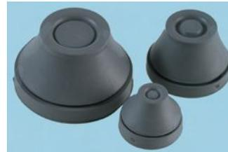
EPDM is generally more resistant to cold temperature, diluted acids and ozone than CR material. These products provide an economical alternative to cable glands when taking through a bulkhead or panel. They are quick and easy to install from one side only (no tool is required) and they also provide a measure of cable retention and sealing to IP67 in accordance with EN60529.
