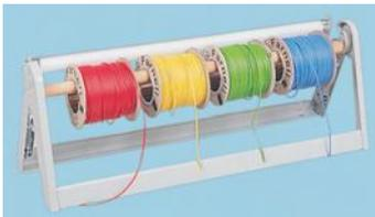
Manufactured from pressed steel with an 18mm wooden cable reel support rod. The reel holder is suitable for either bench or wall mounting. Screw holes are revealed by removing four rubber feet. A sprung foam edged tension bar prevents the cable from reeling out excesses of cable. Supplied with five hardboard reel separators.
