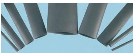
This is a flexible, flame retarded heat-shrinkable polyolefin tubing, with a shrink ratio of 4 : 1 with a thick wall adhesive which melts and flows, to seal components contained within. Recommended for applications requiring water-proofing for light cable and wire harnesses and protection of connector components.
