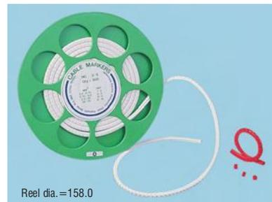
A range of right-facing chevron cut soft PVC cable markers available in either **CEGB** approved black on white or colour coded versions. Supplied semi-severed on self-grip dispenser reels of 1000. Flame retardant to **UL94V-0**.
