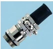
SKINDICHT® SRE are cable glands for screened cables. The earthing sleeve pushed under the braiding ensures a reliable IP protection and EMC compliance. The neoprene sleeve guarantees sealing and kink protection, the cleat provides reliable strain relief.
