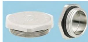
Brass blind plugs with a metric thread for ensuring IP68 protection for unused borings.
