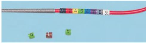
An expandable gusset cable marker manufactured in plasticised PVC. The expanding gusset allows one marker to span a wide range of diameters. Each numeric marker is colour coded and marked with the corresponding number (0-9). Alphanumeric and symbol markers are white and have the legend marked in black. Applicator tools available to fit sizes Z7, Z11 & Z13.
