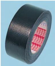
Heavy duty, cloth backed adhesive tape with high tack adhesive for use where normal PVC tape would lose adhesion due to the ingress of water. Often used to fix cables to floor/walls etc. and for general repairs. Supplied on 50m rolls. 50mm wide. Shrink-wrapped for easy storage and display.
