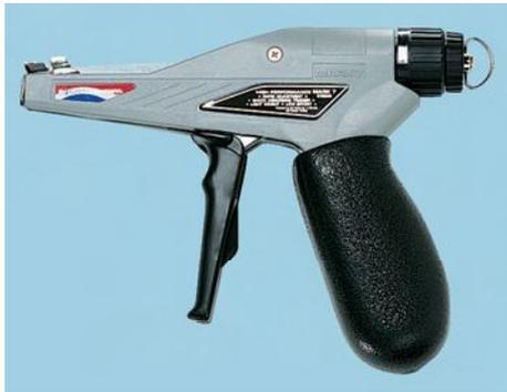
The MK7 Cable Tie Installation Tool with its ergonomic design can be used anywhere. The casing is made of glass fibre reinforced polyester making it extraordinarily light. The MK7 is a state of the art tool for applying HellermannTyton cable ties up to a width of 4.8mm. The MK7 has a three level preset tension device for quick adjustment. Further adjustment is possible within each level. MIL approved.
