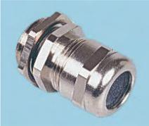
A range of high strength compression glands manufactured in nickel plated brass with either PG or Metric thread. Fully insulated Neoprene cable seal and Pebunan O-ring seal on external fixing thread provide protection to IP68.
