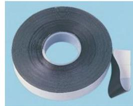
A conformable self-amalgamating tape based on ethylene propylene rubber (EPR) in two widths, 19mm or 25mm. Suitable for jointing and repairing a wide range of power and distribution cables. Can also be used for corrosion protection and water-proofing of many electrical components. The tape conforms to **BS3924** and **IEC454**.
