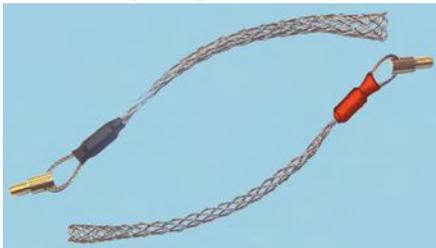
Designed to provide a quick solution for attaching cables and pipes to the Cable Rod. Gripping the object (6 to 10mm) from the outside, and tightening the grip under tension, these socks provide a very reliable, super fast method for securing pipes or cables to the rods.
