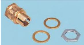
Light duty industrial brass compression glands intended for use with flexible braided power control cables, e.g. 'CY' or 'SY' types. Supplied in two gland kit form comprising two glands, braid clamp washers, galvanised steel locknuts and cable entry seals providing protection to IP66.
