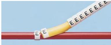
Snap-On Cable Markers allow for the marking of in-situ wiring or cables after termination. Markers are easily and quickly applied using the built-in applicator. The material used to produce the markers is very elastic which allows them to grip the wire and remain in place once applied.
