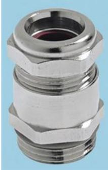
The SKINDICHT® SHV-M-VITON® cable gland is a water proof special gland. The special conical sealing element of VITON® extends through the entire gland and thus guarantees excellent resistance to pressure and strain relief. The VITON® sealing cone is of outstanding resistance to oils and biological oils, solvents and chemicals at high temperatures.
