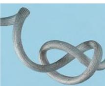
Helaglass is a glass fibre braid lightly impregnated with silicone. Designed to be used for the insulation of wires in heating elements and other domestic appliances subject to high temperatures. This flexible glass-fibre braided slewing is impregnated with silicone and is especially suited for thermal protection in lighting applications.
