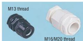
A range of Nylon 66 compression glands complete with lock nut and soft Nylon washer. Designed for use with circular PVC and rubber cable the gland provides a watertight entry and strain relief to IP66. Available in Black or White.
