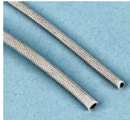
High temperature resistant, silicone impregnated glass fibre slewing ideal for protecting against radial heat. Applications include lighting, domestic appliances, electrical motors and general wiring harnesses. Supplied in 5m cut lengths.
