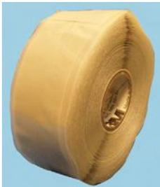
Scotch 70HDT is a high-temperature arc-and fire-resistant tape. This product is just like the Scotch 70 Tape, but has a triangular tapered edge profile (thicker in the middle) and a blue guideline to make half-lapping application easier. Scotch 70HDT has a peak thickness of 20mm, and an edge thickness of 8mm. It is available in a roll size that is 25mm x 9.14m, with a 25mm core.
