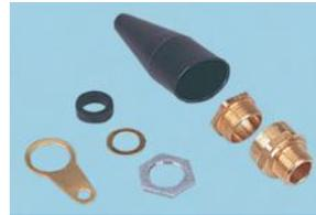
Industrial brass compression glands manufactured to BS6121 Part 1 requirements, for use with all types of unarmoured cables requiring a waterproof outer seal. Supplied in two gland kit form comprising two glands, galvanised steel locknuts, PVC shrouds and cable entry seals providing protection to IP66.
