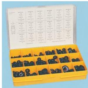
A kit of 18 different sizes of grommets suitable for use with 1.6mm thick panels. The kit covers a range of panel hole sizes from 4.8mm to 20mm, with cable hole diameters ranging from 3.2mm to 15.9mm. Supplied in an 18 compartment storage box.
