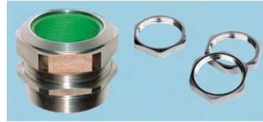
The SKINDICHT® CN-M is a chromium nickel steel cable gland with metric connecting thread and VITON® seal, specially designed for use under tough conditions, e.g. in the pharmaceutical, petrochemical industry (aggressive media) as well as offshore-, dairy- and food area. Suitable counter nut SKINDICHT® SM M CrNi.
