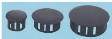
Hole plug in black Nylon 66. Push fitting to blank unwanted holes. To fit panel thickness 0.8mm to 3.2mm. Flame retardant to **UL94V-2**.
