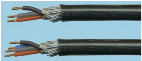
Designed for mains supply electricity. This range of cable is suitable for outside and direct burial. XLPE offers advantages over both PVC and Polythene, notably in its ability to allow greater current carrying capacity, higher overload and short circuit performance.
