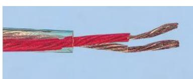
A superb quality, flexible two core twisted speaker cable with 189 strands of 99.99% oxygen free copper (OFC) conductors that ensures high precision music transmission and crystal clear, crisp sound quality. The conductors and cable are sheathed in transparent PVC. Supplied on 100m reels.
