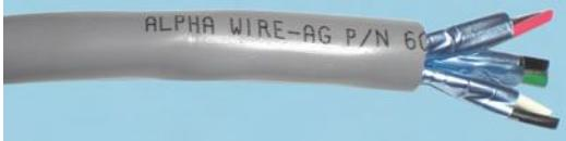
Alpha-Byte™ Low Capacitance Data Cables have improved transmission characteristics and are suitable for extended distance transmission. The unique structure of these cables enable the cable pairs to exhibit a lower dielectric constant - resulting in less loss, lower signal distortion and higher transmission speeds. Suitable for use with EIA RS-232C, RS-422, RS-423 and RS-449 interfaces.
