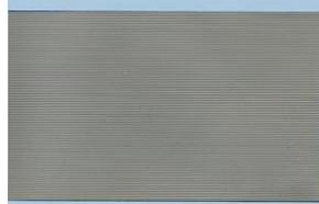
The 0.635mm (0.025") grey PVC insulation flat ribbon cable is used with 3M P25E 1.27mm (0.050") sockets, 82xx-600xx sockets and all other cable mounted connectors on 1.27mm pitch. 30AWG stranded conductors provides flexibility and extended life. The cable is zippable for branching or discrete termination.
