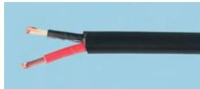
Insulated wires manufactured to BS6862 Part 1 for automotive, marine and agricultural applications. PVC insulated, plain annealed copper wire resistant to petrol, lubricant oils, fuel oils and dilute acids. Supplied in 100m reels.
