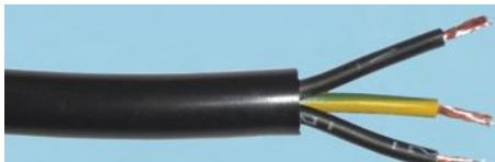
OLFLEX® Classic 110 Black 0,6/1 kV cables are control and connecting cables with a black outer sheath for use in dry, damp and wet rooms, for normal mechanical abuse. At ambient temperature it is generally resistant against acids, caustics solutions and certain oils. Continuous movements or usage of these cables in moving cable carriers or on motor drum guidance or under a strain of more than 15 N/mm<sup>2</sup> is not allowed.
