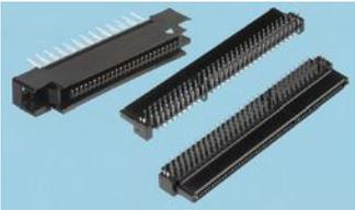
For generic use across applications in many electronics markets the 1.27mm (0.050") cable mount IDC sockets assemble to either 0.635mm (0.025") or 1.27mm (0.050") flat ribbon cable. Mating through-hole plated boardmount plug connectors allow for wire-to-board applications. Also features board-mount sockets and plugs to satisfy board-to-board applications.
