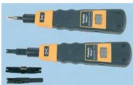
Terminates and cuts telephone wire and data cable. Removable blades for cabling into 110 and Krone LSA panels. The tool will accept all manufacturers twist and lock blades. Within the handle the adjustable impact force control ensures that the tool meets the demands of all cables. Also fitted to the handle are two tools, a hook to feed wires through holes and a multi use spudger: screwdriver and IDC contact insertion tool.
