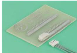
0.8mm pitch IDC connector system for wire to board applications
