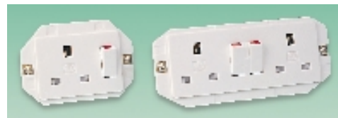
107-723 1 Gang Panel cut-out: H = 48.4, W = 68.2, Corner radius = 2.8, Fixing centres = 80.0, Rear projection = 23 107-724 2 Gang Panel cut-out: H = 48.4, W = 124.6, Corner radius = 2.8, Fixing centres = 136.0, Rear projection = 23
