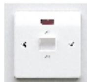
30A DP Switch + Neon H = 86, W = 86 Fixing centres = 60.3
