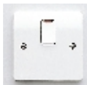
20A DP Switch + Neon H = 86, W = 86 Fixing centres = 60.3
