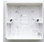
30mm Box H = 87, W = 87 (2 gang = 148) Fixing centres = 60.3 (2 gang = 120.6)
