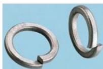
BS 4464 Type A mild steel single coil spring washers. As the spring is compressed it exerts a locking pressure on the nut. Bright Zinc plated.
