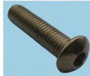
ISO 7380 Grade A2 (18/8) Stainless Steel precision manufactured fastener. Button head with hexagon drive. Corrosion resistant under normal atmospheric conditions.
