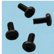
Din 7985 grade 4.8 mild steel machine screws. Cross-recessed drive with a pan head, fully threaded. Chemically blacked finish.
