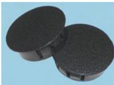
This nylon dome plug is ideal for covering unwanted openings, with its convex, matt finished head tapering to a thin edge for an excellent appearance. As the dome plugs are manufactured from nylon 6,6 they offer a good resistance to most solvents, aromatic hydrocarbons, dilute alkalis, detergents, oils, greases, and fats. They also offer a limited resistance to dilute acids and offer a short term working temperature
