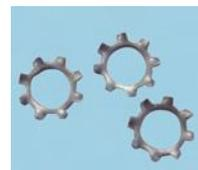
Din 6797 mild steel external toothed locking washers. Under locking pressure the teeth are forced into the mating product to provide a locking feature. Bright Zinc plated.
