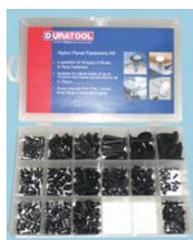
This kit contains a selection of 18 types of nylon rivets and panel fasteners suitable for panel holes of up to 10.0mm and panel combinations of up to 33mm. Styles include the pine tree, the canoe, the push rivet and the drive rivet.
