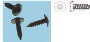
Mild steel self tapping screws. Recessed pan head, type AB (gimlet point). Will tap and form their own threads into mating material. Chemically blacked.
