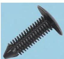
This nylon pine tree clip with its triangular point will securely hold wood, particle board, metal, solid or foam plastic, and rubber panels. It is quick and easy to install and can be used with threaded or non-threaded holes as well as in blind hole assemblies. The clip has a patented twist-in multiple head design for blind mounting of panels, and has a 360° anchoring surface to provide a stronger hold on thin materials.
