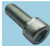
Din 912 Grade 12.9 high strength steel precision manufactured fastener. Cap head with hexagon drive. Can be used in critical applications where service load is high. Bright Zinc plated.
