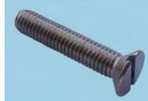
Din 963 Grade A2 (18/8) Stainless Steel machine screws. Slotted drive with a countersunk head, fully threaded. Corrosion resistant under normal atmospheric conditions.
