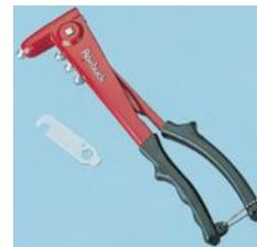
Designed for setting blind rivets of all diameters in all groups except 5mm 3/16in where use is restricted to alu group rivets. Forged steel drive handle with pressure cast body. Self-opening, with alloy steel jaws and spare nozzles screwed into the body.
