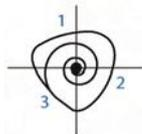
**Tri - Lock™ Threadform.** Three flats on thread means less surface contact between screw and material when driven in.
