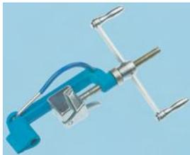
The Band-It tool is a drop forged, electroplated tool with tensing capability of over 2,400lb with built-in cutter. (Caution: Operator can exceed bands breaking strain with this tool).
