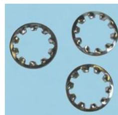
Din 67975 mild steel internal toothed locking washers. Under locking pressure the teeth are forced into the mating product to provide a locking feature. Bright Zinc plated.
