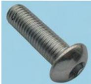
ISO 7380 Grade 10.9 high strength steel precision manufactured fastener. Button head with hexagon drive. Low profile head is suitable where safety (no sharp edges or protrusions permitted) may be an issue.
