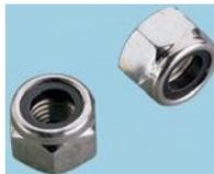
Din 985 Grade A2 (18/8) Stainless Steel self locking nuts. The nylon insert resists loosening, working on the principle of thread friction. Corrosion resistant under normal atmospheric conditions.
