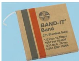
Type 201 stainless steel has superior yield and tensile strength properties to provide maximum clamping strength. All sizes have fully rounded smooth edges for safety and easy installation. For greater strength, use double wrap, threading the buckle each time round. 100 foot coils.
