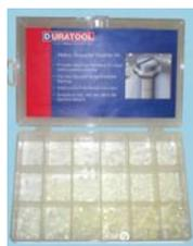
The shoulder washers in this kit provide electrical insulation for metal metric machine screws and help to prevent electrolytic corrosion. They can also be used as lightly loaded bearings. The kit provides washers suitable for machine screws ranging from M3 to M8 in size.
