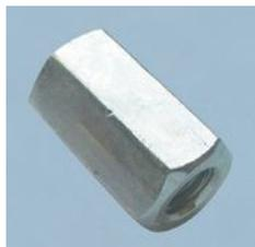
Din 6334 mild steel studding connectors. Can be used as spacers or to connect lengths of studding. Bright Zinc plated.
