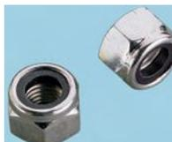
Din 985 Grade A4 ("acid proof") Stainless Steel self locking nuts. The nylon insert resists loosening, working on the principle of thread friction. Better corrosive resistance to aggressive media such as chlorides.
