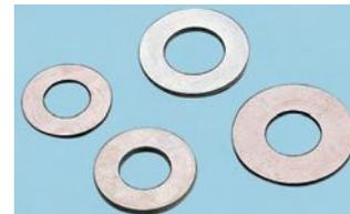
Din 125A Form A Grade A2 (18/8) Stainless Steel washers. Standard washer for protection of mating material and spreading the clamp load. Corrosion resistant under normal atmospheric conditions.
