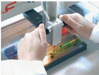
The pick and place station PRECITEC® is a new manual system for the placement of SMT-components. It is a perfect ergonomic station including a lot of functions with an attractive price.
