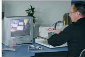
Autonomous visual inspection system. Suits to verify solder paste, glue, different types of fluids and SMD installation before and after reflow.
