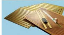
We recommend you to mount the self-adhesive contact strips on a grounding point motherboard (such as RE201-LFDS or RE334-LF) for optimum use and reduction of interference fields.
