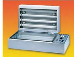
The first double sided UV-exposure unit is an economic version. Nevertheless it is equipped with a vacuum pump and a mechanical timer from 0' to 7'. The boards and film are securely fixed through a clear polyester sheet. Switching of top and bottom lighting can be done separately for the DFE 2340 model.
