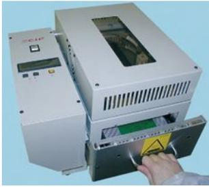
FT02 oven has been conceived to the reflow of solder paste and polymérisation of the glues for prototyping. FT02 oven is compatible with high temperature alloys and above all "lead free" ones thanks to its new heating system as well as its electronics.
