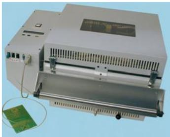
The reflow oven FT05 is a new generation professional oven. It was created to work with the new high temperature alloys, including lead free alloys in force on the 1st of July 2006.
