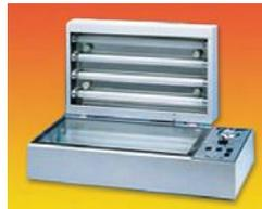
The first double sided UV-exposure unit is an economic version. Nevertheless it is equipped with a vacuum pump and a mechanical timer from 0' to 7'. The boards and film are securely fixed through a clear polyester sheet. Switching of top and bottom lighting can be done separately for the DFE 2340 model.
