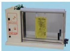
Two models which allows etching, cleaning and developing in a single unit with 3 tanks. A complete clear tank arrangement of 100% welded PVC. Rigid, stable and compact units supplied with two thermostatic controlled heating elements and two air bubble pumps. The Serie GR units allow you to develop prototypes or other to be etched materials in combination with a rinsing tank for DI-water.
