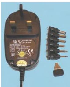
A Regulated plug-in power supply with 7 output voltages. Polarity can be changed by reversing the plug connection. Interchangeable DC plugs with 6 common sizes included.
