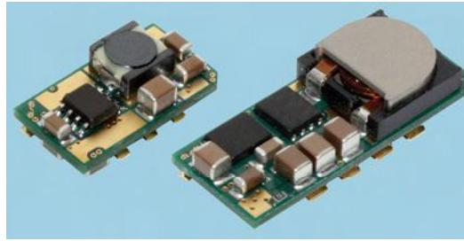
YM Series: H=6.27, W=20.32, D=11.43mm
