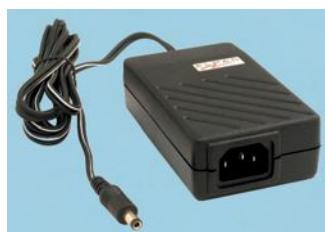
Designed to support medical applications like instruments, patient monitors, and lab equipment, but also portable units. Fully enclosed (polycarbonate case) external AC/DC medical desktop power supply, with switch-mode technologies for DC powered universal applications. Provides 24W of power in fully regulated and protected outputs of 12, 15, 18, and 24 Vdc, with low ripple.
