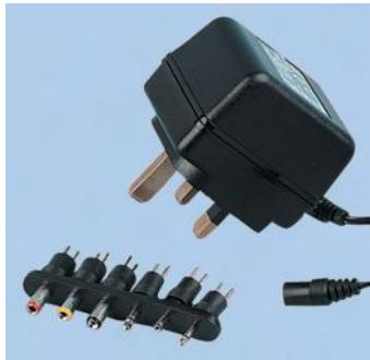
A range of AC/DC mains plug-in power supplies manufactured to BS3535/EN60742. The power supplies give fixed, regulated DC voltage outputs. Supplied with integral 1.8m lead and a set of 6 interchangeable connectors including 4 popular DC type power plugs and 2.5mm/3.5mm jack type plugs. Polarity can be easily changed by reversing the plug connection.
