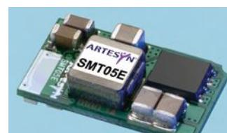
The SMT series are non-isolated DC/DC converters packaged in a surface mount footprint. The SMT is designed for applications including distributed power, workstations, optical network and wireless applications. Implemented using state-of-the-art surface-mount technology and automated manufacturing techniques, the SMT offers compact size and with a high efficiency.
