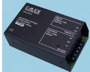
High quality unregulated, chassis mounting power supplies. All models use rugged screw terminal blocks for input and output connections. The metal case provides screening and threaded inserts allow these supplies to be mounted on the insulated Tufnell® base or on the side. Outputs can be short circuited for a maximum of 3 minutes. These models use toroidal transformers to reduce magnetic fields and have fused output protection.
