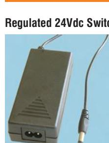
A 65W desktop, switch mode, regulated 24Vdc UK plug-in power supply. It has a 2pin AC inlet and 1.8m output lead fitted with the popular right angled 2.1x5.5x12mm centre positive connector. The connector used is the right angled type, which helps to reduce risk of accidentally unplugging the unit.
