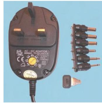
A non-regulated plug-in power supply with 6 output voltages. Polarity can be changed by reversing the plug connection. Interchangeable DC plugs with 6 common sizes included.
