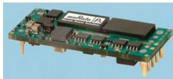
The UCE series offers fixed output voltages from 1.5 to 12 Volts and currents up to 40 Amps. Interleaved synchronous rectifier topology yields excellent efficiency over 90% and no reverse output conduction. These converters offer tight output regulation and high stability even with no load. The unit is fully protected against input undervoltage, output overcurrent and short circuit. An on-board temperature sensor shuts down the converter if thermal limits are reached.
