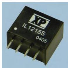
A new low cost range of 2W isolated dc/dc converters. The IL series comes in one of the smallest packages available today and has single outputs ranging from 5 Vdc to 15 Vdc with inputs of 5 or 12 Vdc. The units are available in a SIP package style and feature short circuit protection.
