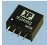
A new low cost range of 1W isolated dc/dc converters. The IE series has single outputs ranging from 5 Vdc to 15 Vdc with inputs of 5, 12, or 24 Vdc. The units are available in both SIP and DIP package styles and feature short circuit protection.
