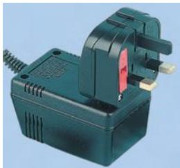
Useful mains adaptors allowing 2-pin European plug-in power adaptors to be used with UK sockets. The adaptors feature specially designed pads to grip onto the plug body of power adaptors for a secure attachment, the pads are engaged by tightening two screws and maintain their integrity over time.
