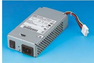
A new Low Power unit designed to address the needs of networking product manufacturers. With a low profile design that can fit in 1U rack configurations, the new LCT43-E model accepts universal AC input (85 to 264VAC and 120 to 370VDC) and has triple DC outputs of 5V, +12V, and -12V. The unit provides 47W of output power with 12 CFM forced air.
