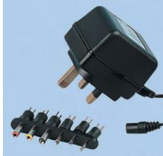
A range of AC/DC mains plug-in power supplies manufactured to BS3535/EN60742. The power supplies give a fixed DC voltage outputs. Suitable for general purpose audio/video and computer equipment. Supplied with integral 1.8m lead and a set of 6 interchangeable connectors including 4 popular dc type power plugs and 2.5mm/3.5mm jack type plugs. Polarity can be easily changed by reversing the plug connection.
