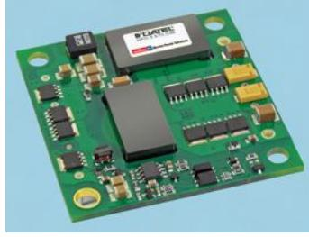
Using both surface-mount technology and planar magnetics, these converters are manufactured on lead-free, open-frame packages with an industry-standard pinout. These converters utilize a full-bridge, fixed-frequency topology along with synchronous output rectification to achieve a high efficiency. Features also include input undervoltage shutdown circuitry, output overvoltage protection, output short-circuit and current limiting protection and thermal shutdown.
