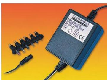
A range of AC/DC in-line, mains power supplies manufactured to European standards. The power supplies operate from a 230V ac, 50Hz mains outlet and give a regulated DC output suitable for various audio/video and computer equipment. The power supply has an integral 2m mains lead, terminating in a 2-pin European plug and 1.8m DC power lead with a set of 6 interchangeable power plugs. A polarity changer is also included.
