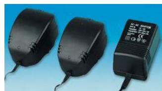
A range of high quality, AC/DC linear mains plug-in power supplied manufactured to BS3535/EN60742. The power supplies operate from standard 230V ac mains voltage and give stepped down, regulated outputs. Termination is via single, fixed 2.1mm or 2.5mm DC power type plugs which is most common type found on audio/video and computer equipment.
