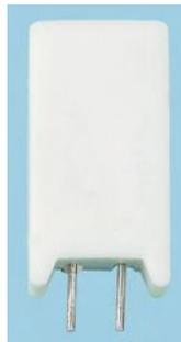
A high purity ceramic rod, with force fit end caps onto which is wound a wire element: or a deposited metal oxide film (depending on value). The element is fitted into a ceramic case with fireproof insulation cement.
