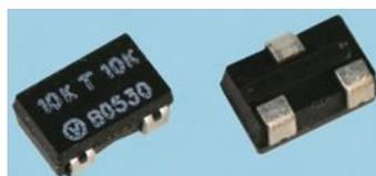
The DSM surface mount divider provides a matched pair of Bulk Metal® Foil Resistors in a small epoxy molded package. The electrical specification of this integrated construction offers improved performance and better real estate utilization over discrete resistors and matched pairs.
