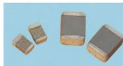
Surface mount PTC thermistors with silver terminations supplied on tape and reel, suitable for **reflow soldering** only. The very small 25V B59701 Series are for limit temperature sensing, and the 80V 120°C B59707 device is suitable for overcurrent protection, time delay and current stabilisation.
