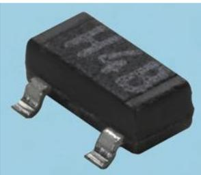
Vishay Thin Film MP Series Dividers provide  $\pm 2$  ppm/ $^{\circ}$ C tracking and a ratio tolerance as tight as  $\pm 0.05\%$ , ultra small size, 3 or 4 lead package and exceptional stability for all surface mount applications. The standard SC70 package format with common standard resistance values provide easy selection for most applications requiring matched pair resistor elements.
