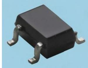
The MPDA Series dividers provide  $\pm 2$  ppm/ $^{\circ}$ C tracking and a ratio tolerance as tight as  $\pm 0.05\%$ , small size, and exceptional stability for all surface mount applications. The standard SOT-143 package format with unity and common standard resistance divider ratios provide easy selection for most applications requiring matched pair resistor elements.
