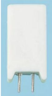
A high purity ceramic rod, with force fit end caps onto which is wound a wire element; or a deposited metal oxide film (depending on value). The element is fitted into a ceramic case with fireproof insulation cement.
