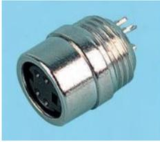
An S-Video type (4-pin MiniDIN) socket with solder bucket terminations. Supplied with fixing nut. Panel cutout:  $\varnothing$ 11mm approx.
