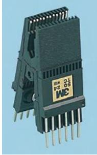
These test clips are for the easy and convenient testing of surface mounted small-outline IC's (SOIC's). Strong helical springs and insulating contact combs ensure contact integrity during testing. Probes or single row female connectors will connect to the 0.025" (0.63mm) square, gold plated contacts on 0.1" (2.54mm) centres.
