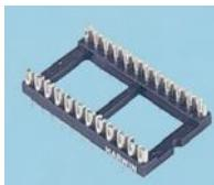
Slotted DIL headers with precision turned contacts, for use in either board-to-board interconnection or for mounting small discrete components. May be used with corresponding DIL socket. Body is black glass filled polyester, UL recognised, contacts are brass with tin on nickel finish. Pin spacing 0.1" (2.54mm). Operating temperature range -55°C to +150°C.
