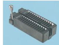
Range of ZIF sockets which will accept DIL devices with 0.3" (7.62mm) to 0.6" (15.24mm) row spacing, with a pin width of 0.38mm to 1.14mm. Sockets are lever locking, ON in DOWN position. Body is of polyphenylene sulphide. 113-6788 is for SO-IC packages
