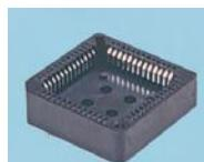
Industry standard sockets for JEDEC A/B PLCCs, incorporating internal standoffs for precision chip positioning, bottom standoffs for simpler flux residue removal, and 2.54mm grid solder tails. **UL** recognised.
