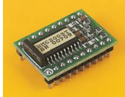
PCB = 27x9, Pin spacing = 2.54x15.24
