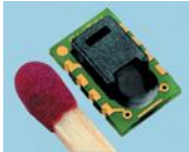
SHT 11 & 15 H = 3.1, W = 5.08, D = 7.62mm
