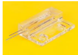
607-265: L=30, W=20, D=7, Pin L=20, Fixing slots=6x3.3. Fixing centres 16 Long lead to top
