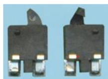
A horizontally actuated detector switch with one NO contact. The switch has a side push of 2.15mm with a 40gf to operate. Available with either left hand or right hand operating direction.
