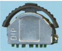
This series of 3 way navigation switches has an integrated centre push switch. They have an electrical life in excess of 100,000 operations. The MCPLJ switch requires an operating force of 40gf on the return actuator and 150gf on the centre push switch. The MCPLS series requires 70gf on the return actuator and 200gf on the centre push switch. MCPL3-AC-V switch has an integrated Mounting Knob.
