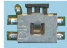
A horizontally actuated TACT switch with one NO contact. The switch has a side push of 0.3mm with a 220gf to operate and a very small PCB footprint. Available with (947-1987) or without (131-6979) Locating Posts.
