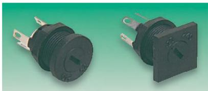
Body: L=14.3, Panel cut-out=12.75 dia, Bezel: Round=15.9 dia, Square=15.9 x 15.9, Keyway=2.54 x 1.25, Tabs L=7.9, W=2.8
