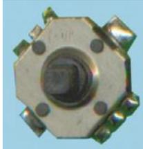
These multidirectional navigation switches require an operating force of 160gf with a centre push of 320gf. They have a very long electrical life of at least 100,000 cycles.
