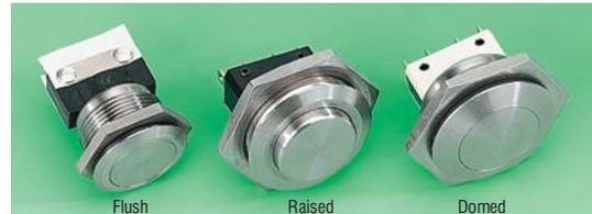
21.5mm L=33.2, Dia=21.5, Depth behind panel=31.6 Max. panel thickness=7.1, Panel cut-out=19.2
