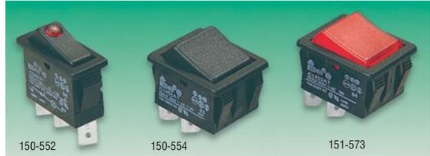
Single pole Bezel=14 x 30.2, Depth=16.2, Panel cut-out=11.5 x 28.2, Tab=6.35 x 0.8
