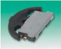
A side-actuated miniature switch with normally open contacts. Rotation of the actuator closes two individual contacts (left or right), while pushing down in the central position closes the two (select) contacts.
