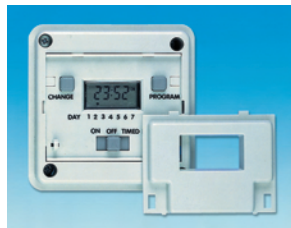
H=72, W=72, D (behind panel)=26 Panel cut-out=67 x 67 (radiused corners 2.5) Terminals=6.3 tabs
