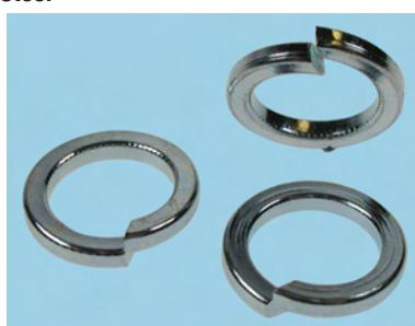
BS 4464 Type A Grade A2 (18/8) Stainless Steel single coil spring washers. As the spring is compressed it exerts a locking pressure on the nut. Corrosion resistant under normal atmospheric conditions.
