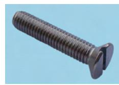
Din 963 Grade A2 (18/8) Stainless Steel machine screws. Slotted drive with a countersunk head, fully threaded. Corrosion resistant under normal atmospheric conditions.
