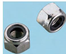
Din 985 Grade 6 steel self locking nuts. The nylon insert resists loosening, working on the principle of thread friction. Bright Zinc plated.
