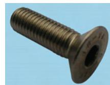
Din 7991 Grade A2 (18/8) Stainless Steel precision manufactured fastener. Countersunk head with hexagon drive. Corrosion resistant under normal atmospheric conditions.
