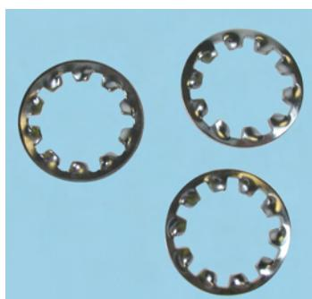
Din 6798 mild steel internal toothed locking washers. Under locking pressure the teeth are forced into the mating product to provide a locking feature. Bright Zinc plated.
