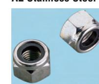
Din 985 Grade A2 (18/8) Stainless Steel self locking nuts. The nylon insert resists loosening, working on the principle of thread friction. Corrosion resistant under normal atmospheric conditions.
