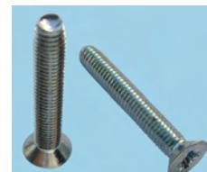
Mild steel recessed countersunk trilobular threadforming screws. Bright Zinc plated and lanolin dipped for ease of application.
