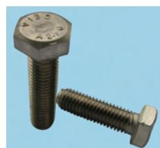
DIN 933 grade A2 (18/8) Stainless Steel multi-purpose set screws. Hexagonal head. Fully threaded. Corrosion resistant under normal atmospheric conditions.
