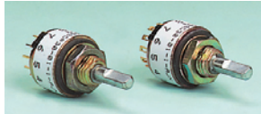
Body: Depth behind panel = 12.9 (solder) 12.37 (PCB) Dia = 12.7 Bush thread = 1/4 28 UNF - 2A Spindle: L = 9.53, Dia = 3.18
