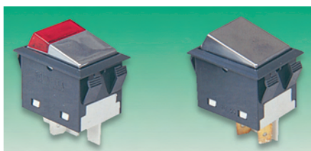
Illuminated Non-illuminated Bezel=35.4 x 27.4, Depth=33.25, Panel cut-out=34.5 x 23.5, Tabs=6.3
