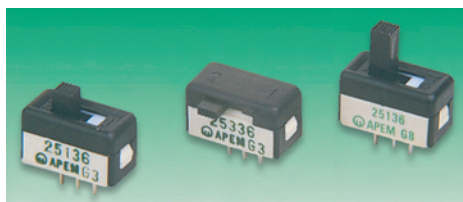
Standard top button H=11, W=14, D=8 (DPDT=12.5)
