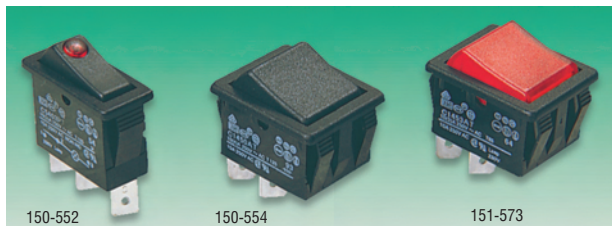
Single pole Bezel=14 x 30.2, Depth=16.2, Panel cut-out=11.5 x 28.2, Tab=6.35 x 0.8 Double pole Bezel=25 x 30.2, Depth=16.2, Panel cut-out=22.3 x 28.2, Tab=6.35 x 0.8
