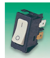
480-344 481-087 Panel cut-out=26.2 x 12.4 (snap-in fixing) Panel cut-out=27.2 x 12.4 (snap-in fixing) Facia=23.8 x 13.1 with 3.4 radius corners Bezel=29.5 x 15.0 Panel thickness=0.75/1.25, Tab=6.3 x 0.8
