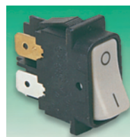
480-344 481-087 Panel cut-out=26.2 x 12.4 (snap-in fixing) Panel cut-out=27.2 x 12.4 (snap-in fixing) Facia=23.8 x 13.1 with 3.4 radius corners Bezel=29.5 x 15.0 Panel thickness=0.75/1.25, Tab=6.3 x 0.8
