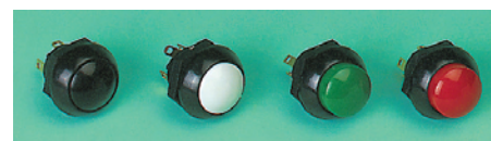
L=21, Dia=17.5 Panel cut-out=11.9 x 11.3 (single flat), depth behind panel=14.0
